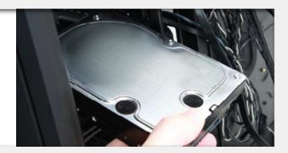
Attach SATA cable and SATA power cables to each hard drive.
