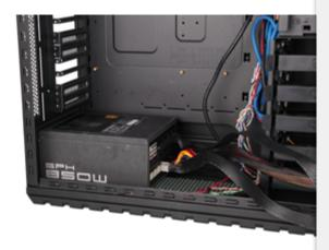
Make sure the power supply is firmly in place, and pushed all the way against the back of the case. Secure it to the case with the screws that came with your power supply.
